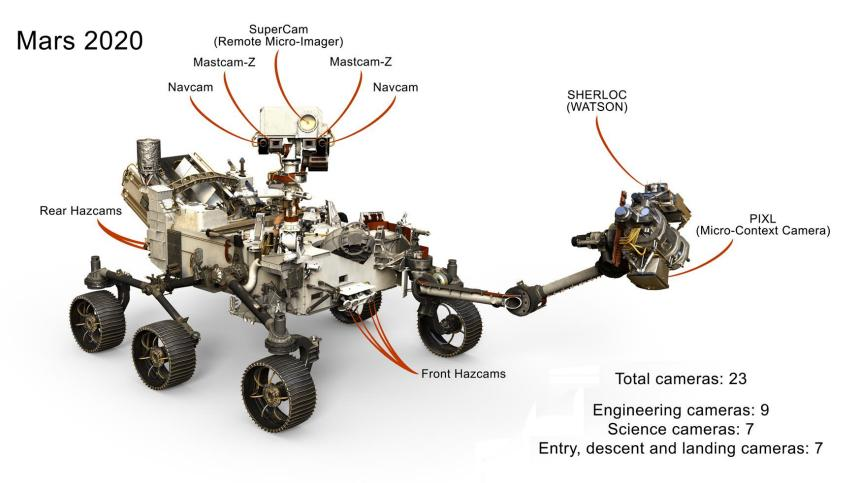
NASA's Mars 2020 mission will have more "eyes" than any rover before it: a grand total of 23, to create sweeping panoramas, reveal obstacles, study the atmosphere, and assist science instruments. They will provide dramatic views during the rover's descent to Mars and be the first to capture images of a parachute as it opens on another planet. There will even be a camera inside the rover's body, which will study samples as they're stored and left on the surface for collection by a future mission.
